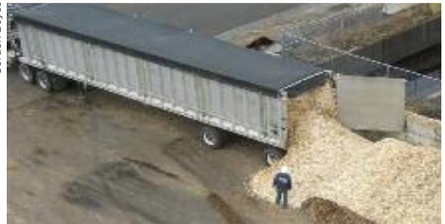
A trailer of biomass being unloaded at a power plant
